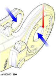
Lift the parallel arm, lower it and put it in mounting position with the lower arm.
